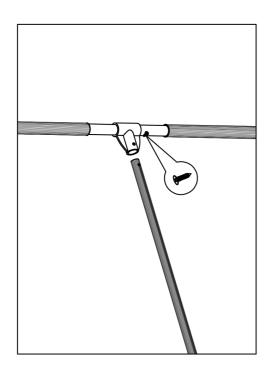
2. Use st3\*10 pan head screw to fix the bar and hanger rod
