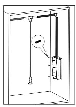
1. Use12 pcs st4\*20 sink head screw to fix the buffer system according to schematic diagram of installation
