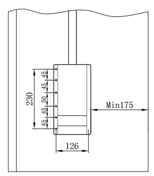
Schematic diagram of installation dimensions (the location indicated the position of screw showed in step 1)
